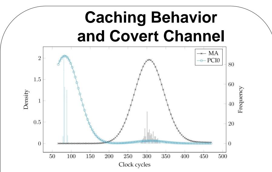
The blue line in this figure is the distribution of CPU memory access latency when accessing cache lines recently written by the FPGA; a typical distribution is shown in black. Our measurements show that cache lines written by the FPGA are placed in the last-level cache of its host CPU.
