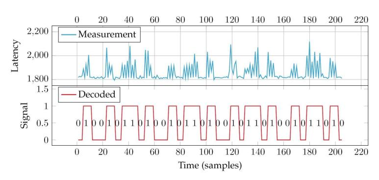
We constructed a covert channel with the FPGA as the sender and a cooperative CPU program as receiver. The FPGA sends binary messages by writing to a cache line when transmitting a 1 and staying quiet otherwise. The receiver continuously probes a the cache set to detect access latency fluctuations to receive the messages. An example decoding of the latency measurements is shown in the figure above. While using heavily redundant encoding, we still achieve a **throughput of 94.98 kBit/s**.
